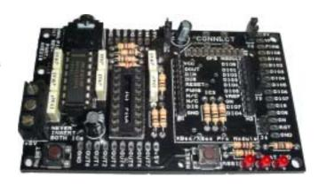
Whilst the 433 modules are low cost and may be suitable for some very simple PICAXE applications, the XBee modules offer considerable advantages. The primary advantage is that the XBee modules are 'bi-directional'. Most budget 433 systems only transmit in one direction, so the transmitter has no idea whether the receiver is actually getting the data! The XBee modules transmit and receive in both directions, so you can easily test (at both ends) if the system is working correctly.
