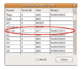
The 'Close' button will close the Debug screen when calibration of the sensor has been completed and allows editing of the PICAXE Basic program to continue.
