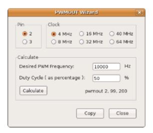
First, select the output pin on which PWM will be generated and choose the operating frequency the PICAXE will be using. Available options will be presented according to the PICAXE type being used. The PICAXE type can be changed using the Options settings described earlier.
