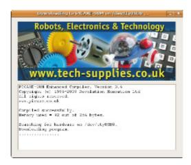
After programming completes a status message will be produced providing information about the programming and PICAXE firmware as appropriate or the Debug Display will automatically launch if the program contains a debug command.
