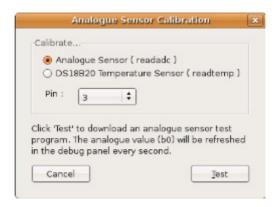
First, select whether it is an analogue sensor or a DS18B20 temperature is to be calibrated, then select the pin to which the sensor is connected.
