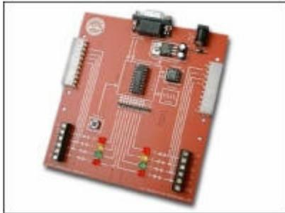
To upgrade the system simply remove the old 18 pin chip in the centre of the Stamp Controller and replace with the new PICAXE-18M2-ST chip, ensuring pin1 is at the top of the board. That's it – easy to do in under 30 seconds!
